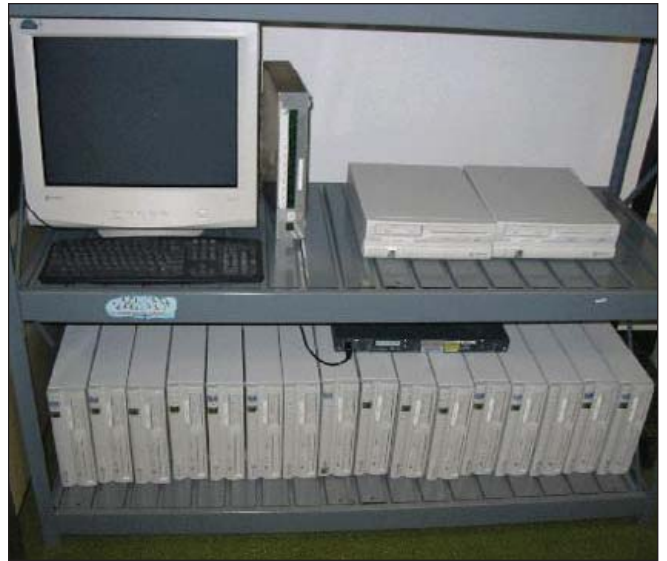
Figure 5. Our cluster, consisting of 17 recycled PCs, improves response times for users' queries.
