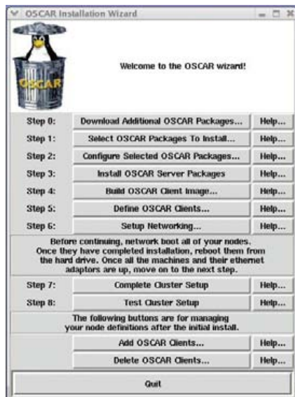
Figure 2. The OSCAR installation wizard lets you deploy, configure and test cluster software.
