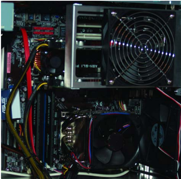
Figure 2. Part of the Cooling Setup for the Ultimate Linux Desktop
