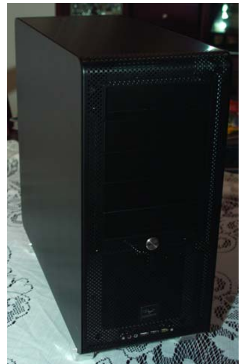
Figure 4. The front panel is along the bottom of the machine. You also can see the mesh mentioned earlier.
