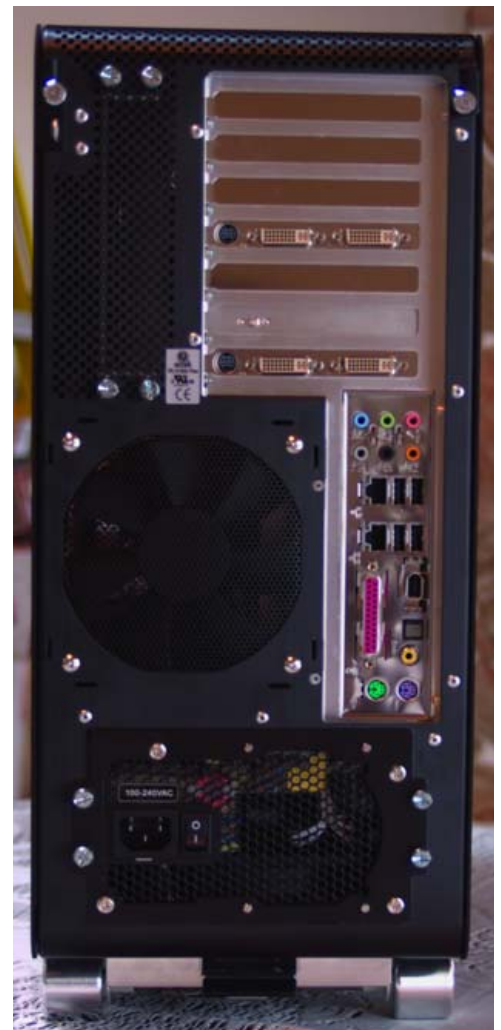
Figure 5. The back panel offers most of the hookups, along with many spots for ventilation, including mesh and cut-outs for fans.
