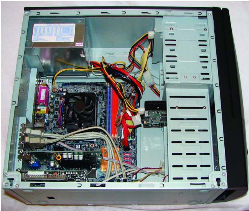
Figure 2. The internals of the Linux Beach MultiMedia Center 500; the motherboard is the same as the LBMC 1000.
