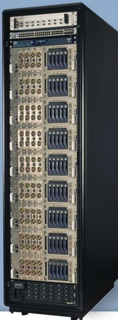
▲ Microway® Quad Opteron™ Cluster with 36 Opteron 880s, redundant power, 45 hard drives and Myrinet™ in our CoolRak™ cabinet.
