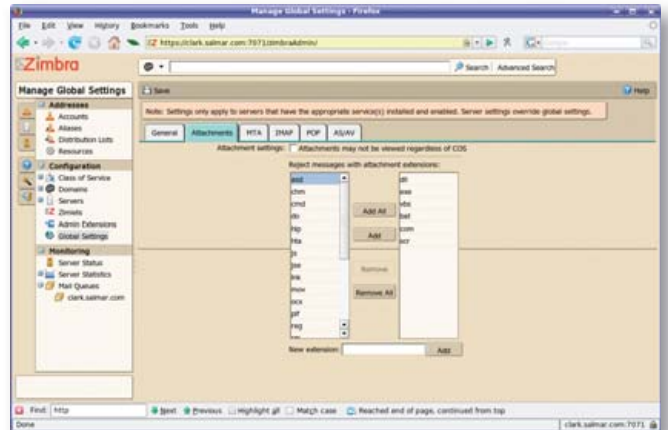
Figure 6. The administrative interface lets you reject messages whose attachments have questionable extensions.
