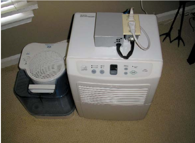
Figure 6. Completed Humidity Controller with Humidifier and Dehumidifier Connected
