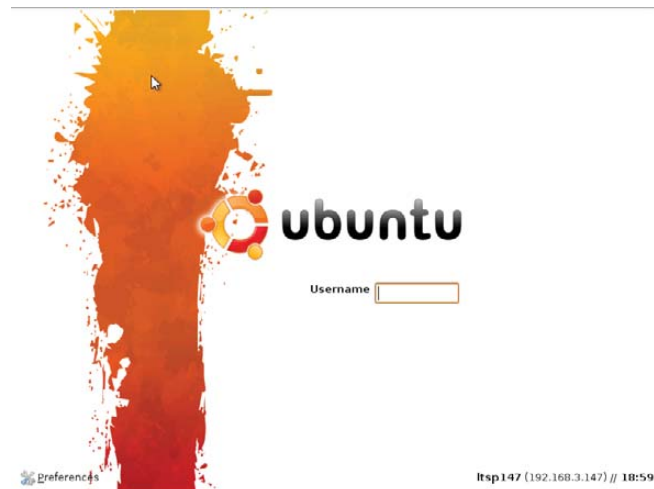
Figure 3. Ubuntu PXE Boot Client LTSP Session (note the lower right-hand corner of the screen)
