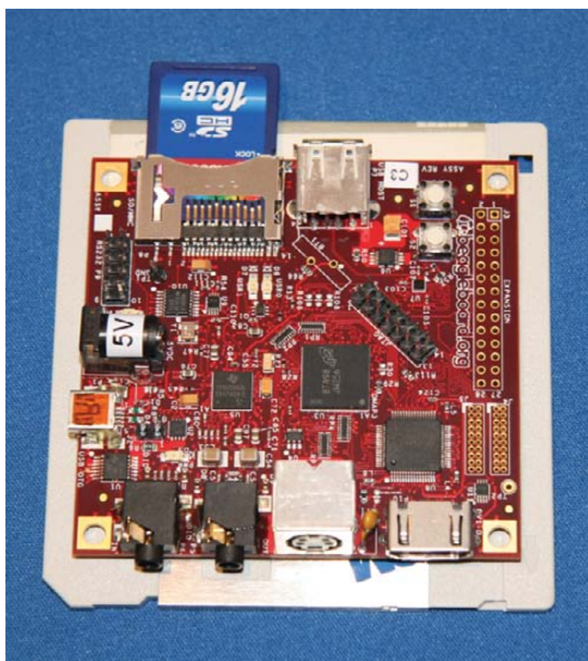
Figure 1. Up close with the Beagle Board—the gray thing underneath it is a floppy disk for scale.
