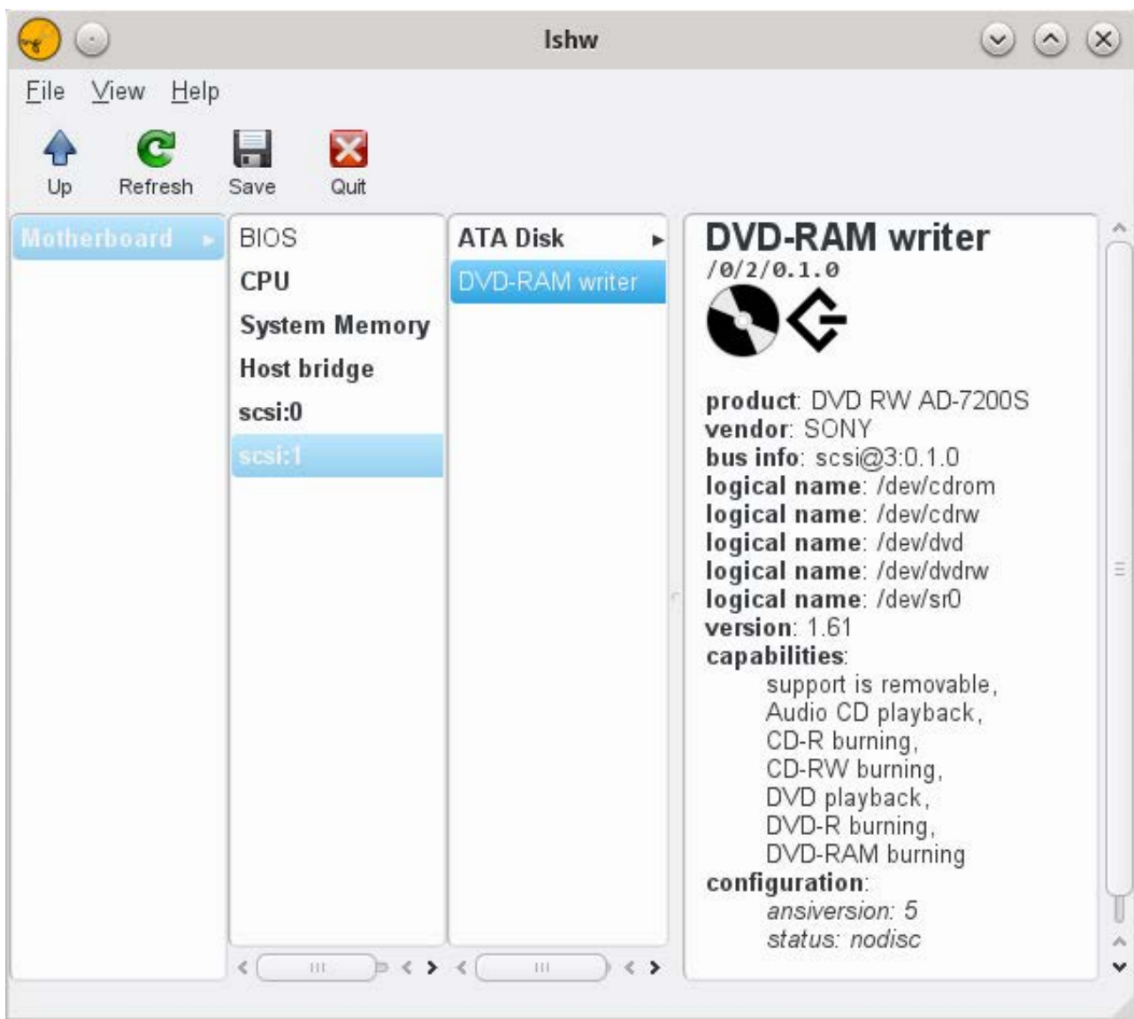
Figure 4. The lshw -X command produces a graphic interface that lets you browse all hardware devices.
