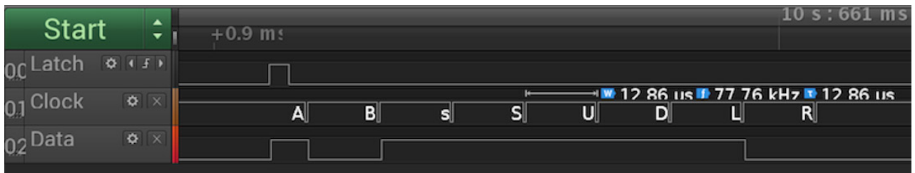
Figure 4. Latch, Pulse (Clock) and Data Line Example
