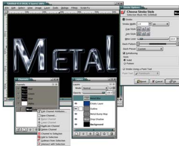
Figure 10. Add a new layer above the bump mapped layer. Open the Channels dialog and click on the channel name for the saved selection. Select Channel to Selection to retrieve the selection. Click on the new layer in the Layers dialog to make it active again. Set the foreground color to gray (#a4a4a4). Open the Stroke Selection dialog (Edit→Stroke Selection) and set the stroke width to 1. Turn off the selection (Ctrl-Shift-A or Select→None). Offset this layer (Layer→Transform→Offset) by 2 pixels in both the X and Y direction. Add a new layer and fill it with blue (#103B82). Set the layer blend mode for this blue layer to Soft Light. Reduce the opacity to 53%.
