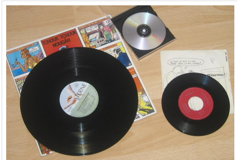
A 12-inch (30-cm) 33 \frac{1}{3} rpm record (left), a 7-inch 45 rpm record (right), which are both analog sound storage mediums, and a CD (above), a digital medium.
